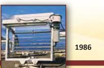
EMMAQUA+®, the next generation of accelerated weathering devices, is introduced. Advancements include individual cycle programming, black panel temperature control, and altazimuth solar tracking for more efficient delivery of full-spectrum solar energy
