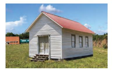
Outdoor weathering testing in a replicated end use environment, like the shed shown above, can demonstrate interactions between components and give a more realistic representation of outdoor product durability.
