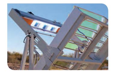
Atlas introduces four patented suites of Temperature-Controlled EMMAQUA. (Static, Night, Dynamic Temperature and Variable Irradiance Control). This breakthrough allows for the testing of materials that are sensitive
