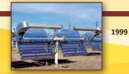
Atlas introduces four patented suites of Temperature-Controlled EMMAQUA. (Static.) Night, Dynamic Temperature and Variable Irradiance Control). This breakthrough allows for the testing of materials that are sensitive to thermal buildup.
