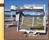
The first EMMAQUA® device, constructed with a wooden frame and sheet metal skin. is patented, manufactured and placed into
