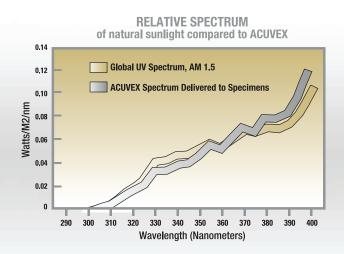
This graph portrays the absolute spectrum of natural sunlight compared to ACUVEX. With the ACUVEX unit, radiation intensity at the specimen surface is much greater than with natural sunlight exposure—providing faster tests.
