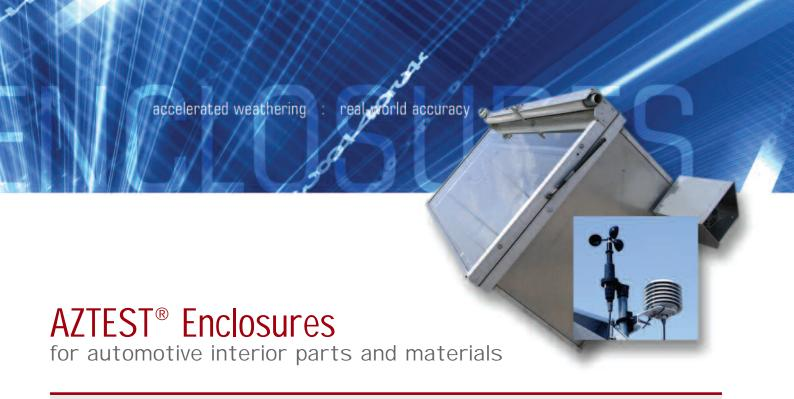
AZTEST Enclosures for Automotive Interior Materials provide vital data and real-world results for interior weathering performance. Automotive interior materials can reach soaring temperatures—exceeding 110° C (230° F) on a summer day in Arizona. Heat and the altered light spectrum from window glass, significantly affects interiors. Add in time, and the effects are both measurable and dramatic.
