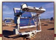
Atlas introduces four patented suites of Temperature-Controlled EMMAQUA. (Static.) Night, Dynamic Temperature and Variable Irradiance Control). This breakthrough allows for the testing of materials that are sensitive
