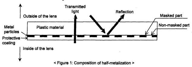
As you see in the figure above, in a microscopic view, the metal particles placed between the plastic and protective coating create partial maskings on the lens, whereas the light passes from the non-masked part only. However, when used in a lamp, this reduced transmission will be balanced out by other designing factors so that the lamp satisfies all the FMVSS108 requirements (e.g. photometric, color) applicable to it.
