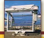
EMMAQUA+®, the next generation of accelerated weathering devices, is introduced. Advancements include individual cycle programming, black panel temperature control, and altazimuth solar tracking for more efficient delivery of full-spectrum solar
