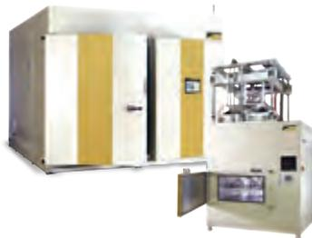
A group of integrated, easy-to-use test chambers for various solar and environmental applications. These instruments combine environmental simulation with metal halide lighting technology and are ideal for testing medium to large sized automotive, plastics, electronics and 3D components, finished products as well as PV modules.
