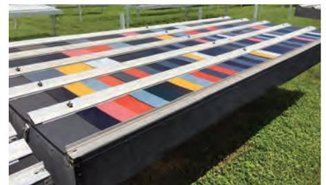
*Other standard outdoor exposure test methods are available, including salt-accelerated, outdoor acid etch, and mildew-enhanced weathering.*
