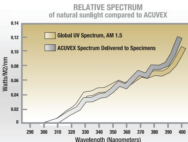
This graph portrays the absolute spectrum of natural sunlight compared to ACUDEX. With the ACUDEX unit, radiation intensity at the specimen surface is much greater than with natural sunlight exposure—providing faster tests.
