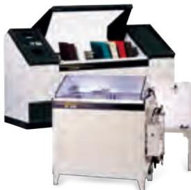
The most sophisticated and versatile corrosion and salt fog cabinets available. Capable of replicating automatic cycling between several environmental conditions to reduce the need to move or otherwise handle test specimens.
