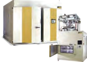
A group of integrated, easy-to-use test chambers for various solar and environmental applications. These instruments combine environmental simulation with metal halide lighting technology and are ideal for testing medium to large sized automotive, plastics, electronics and 3D components, finished products as well as PV modules.
