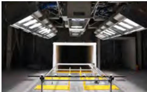
Atlas Custom Systems designs and builds custom solar simulation systems such as walk-in chambers or full-scale test facilities. These full scale test facilities use a series of highly coordinated metal halide lights to provide uniform radiant energy to meet the demanding testing needs of many industries.
