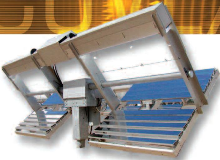
AZTEST's proprietary ACUVEK® for Exterior Materials—Accurate Controlled Ultra Violet Exposure—is an engineered solution that accelerates the effects of material weathering. Its innovative design concentrates sunlight for maximum intensity and measures the related effects on materials.
