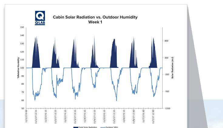
Outdoor weathering testing in a replicated end use environment, like the shed shown above, can demonstrate interactions between components and give a more realistic representation of outdoor product durability.
