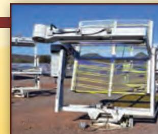
Atlas introduces the UA-EMMA, the latest advancement in outdoor accelerated testing. This device couples the EMMA platform with a new patented mirror system, optimizing real-world correlation.
