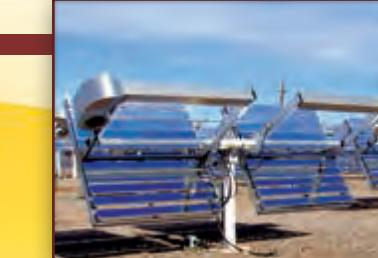
Atlas introduces four patented suites of Temperature-Controlled EMMAQUA. (Static, Night, Dynamic Temperature and Variable Irradiance Control). This breakthrough allows for the testing of materials that are sensitive to thermal buildup.
